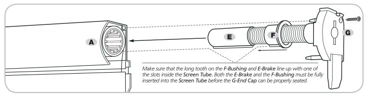
Slip the F-Bushing down the coiled spring to the E-Brake. On the open end of the A-Screen Cassette, insert the E-Brake with F-Bushing into the center of the Screen Tube, aligning the long tooth on both as noted above. Next, match up the large pin on the top of the G-End Cap to the corresponding hole at the top of the A-Screen Cassette Housing. Tap evenly with a soft mallet until the assembly fits snugly.
