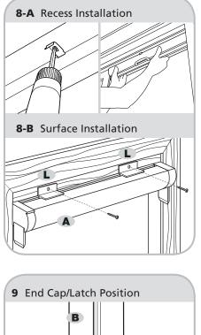
NOTE: It is critical that the Screen Cassette and Rails be installed square and plumb in the door opening. Apply shims (not supplied) as needed.
